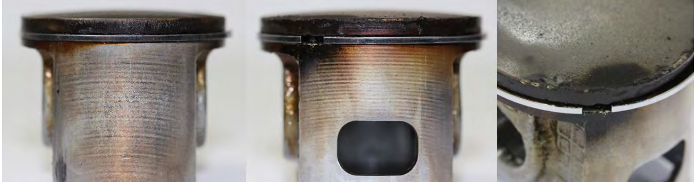
Figure 9: Piston views (150.4 hours + previous ~30 hours)
