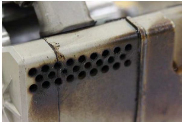
Figure 15: Exhaust outlet (150.4 hours)
