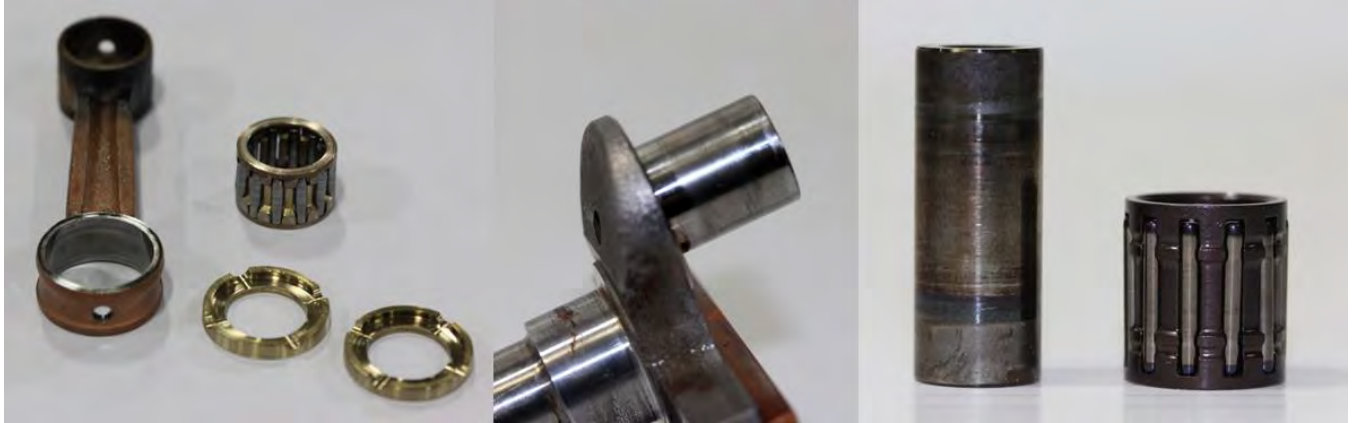
Figure 11: Top and bottom-end rod bearings with rod guides and crankshaft. All components finished the test with no sign of excessive wear. (150.4 hours)
